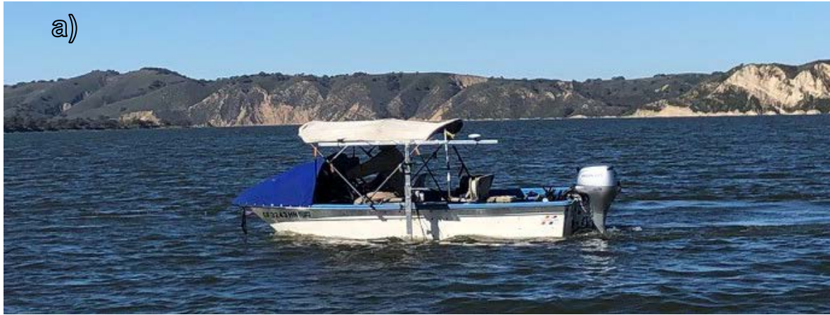
Figure 10: a) multi-beam echo-sounding survey by boat on January 25 & 27 to document final alignment; b,c) survey results for the pipeline alignment, note dredged portion near the intake tower filled in during 1/9/23 storm event (right side of figure b); d) contractor demobilizing working crane utilizing the highest boat ramp (#1) prior to the County re-opening the lake for recreational use following dramatic lake rise.
