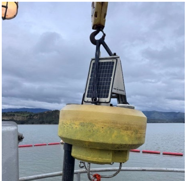
Reinstalled water quality buoy after maintenance work
