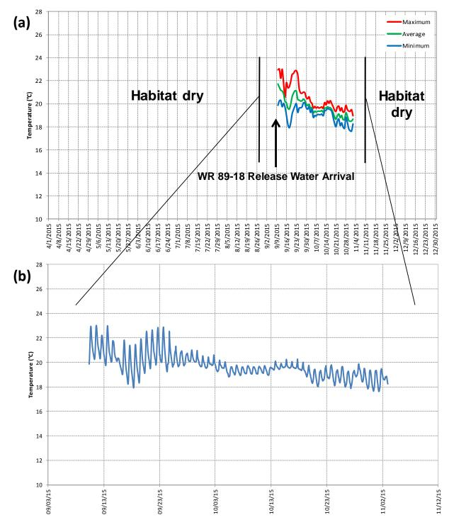
**Figure 15:** 2015 LSYR-4.95 (Encantado Pool) bottom (6.5 feet) thermograph for (a) daily maximum, average, and minimum values and (b) hourly data for the period of 9/10/15 - 11/3/15.
