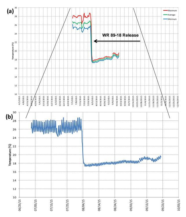
**Figure 6:** 2015 LSYR-0.2 (Stilling Basin tail out) surface (1.0 foot) water temperature for (a) daily maximum, average, and minimum for the entire period of deployment and (b) hourly measurements for the period of record.
