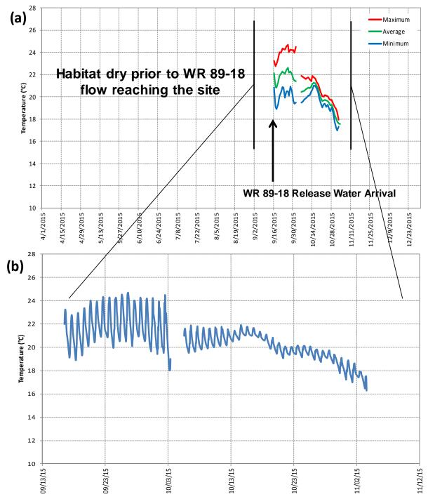
**Figure 22:** 2015 LSYR-10.2 (Alisal Bedrock Pool) surface (1.0 foot) thermograph for (a) daily maximum, average, and minimum daily values and (b) hourly data for the period of 9/16/15 - 11/3/15; the surface unit was out of the water from 10/2/15 - 10/5/15.
