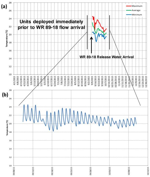
**Figure 16:** 2015 LSYR-7.65 (Double Canopy Pool) surface (1.0 foot) thermograph (a) daily maximum, average, and minimum values and (b) hourly data for the period 9/10/15 - 10/9/15; thermographs were deployed just prior to the arrival of the WR89-18 release.
