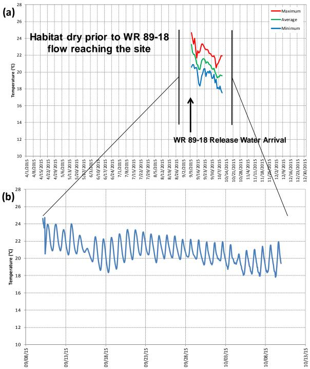
**Figure 19:** 2015 LSYR-8.7 (Head of Beaver Pool) surface (0.5 foot) thermograph for (a) daily maximum, average, and minimum daily values and (b) hourly data for the period 9/10/15 – 10/26/15; habitat unit dry prior to WR89-18 releases.
