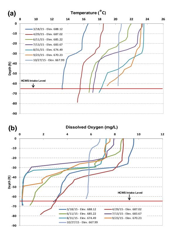
**Figure 42:** Lake Cachuma 2015 water quality profiles for (a) temperature and (b) dissolved oxygen concentrations at the intake barge for the HCWS. HCWS intake hose level was set at 65 feet of depth throughout the monitoring period.
