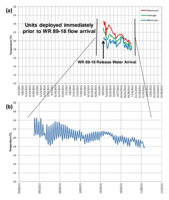
**Figure 18:** 2015 LSYR-7.65 (Double Canopy Pool) bottom (4.0 feet) thermograph for (a) daily maximum, average, and minimum daily values and (b) hourly data for the period 9/10/15 – 11/3/15.
