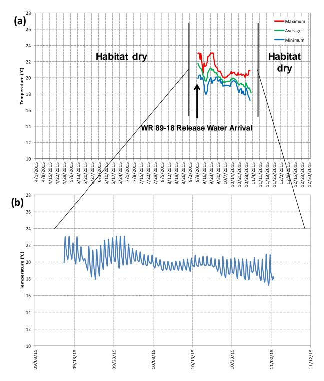
**Figure 14:** 2015 LSYR-4.95 (Encantado Pool) middle (3.5 feet) thermograph for (a) daily maximum, average, and minimum daily values and (b) hourly data for the period of record 9/10/15 - 11/3/15.
