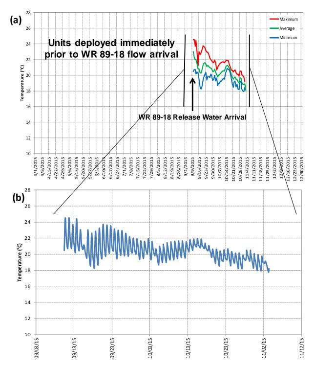
**Figure 17:** 2015 LSYR-7.65 (Double Canopy Pool) middle (2.0 feet) thermograph for (a) daily maximum, average, and minimum daily values and (b) hourly data for the period 9/10/15 – 11/3/15.
