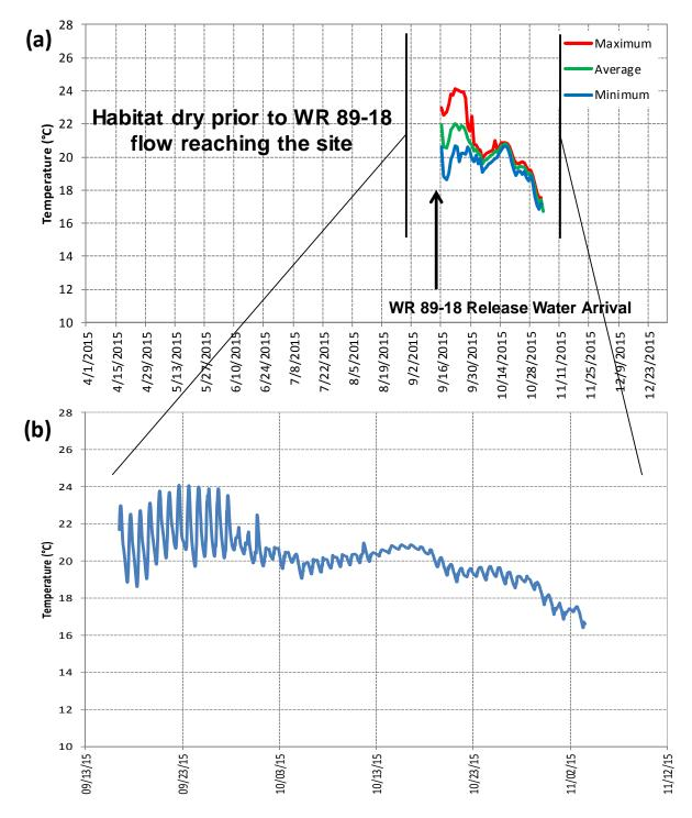
**Figure 23:** 2015 LSYR-10.2 (Alisal Bedrock Pool) middle (4.0 feet) thermograph for (a) daily maximum, average, and minimum daily values and (b) hourly data for the period 9/16/15 – 11/3/15; this habitat was dry prior to the arrival of the WR89-18 release.
