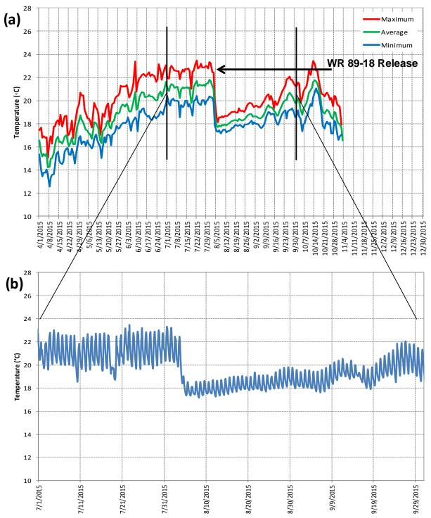
**Figure 12:** 2015 Reclamation property boundary LSYR 0.62 (downstream of the Long Pool) bottom (2.0 feet) thermograph for (a) daily maximum, average, and minimum values and (b) hourly data for the period of 7/1/15 - 10/1/15.
