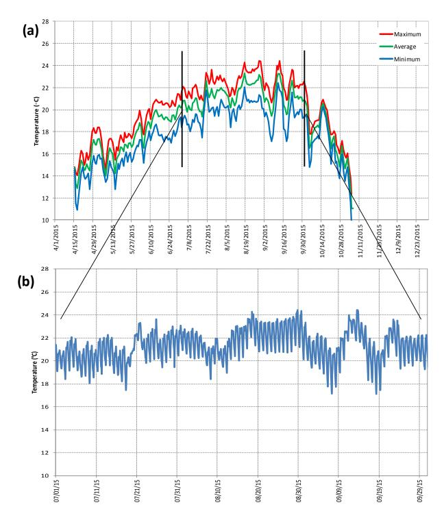
**Figure 40**: 2015 LAC-7.0 (Los Amoles Creek at Ford Crossing) bottom (3.0 feet) water temperature for (a) daily maximum, average, and minimum for the entire period of deployment and (b) hourly measurements for the period from 7/1/15 - 10/1/15; Los Amoles was dry approximately 150 feet upstream of the thermograph location.
