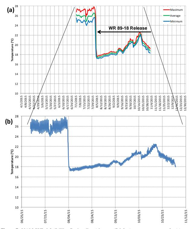
**Figure 7:** 2015 LSYR-0.2 (Stilling Basin tail out) bottom (7.0 feet) water temperature for (a) daily maximum, average, and minimum for the entire period of deployment and (b) hourly measurements for the period of record.
