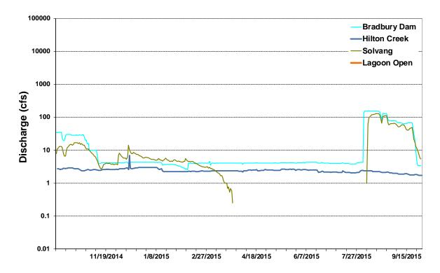
**Figure 3:** Average daily discharge at Hilton Creek, just downstream of the Upper Release Point, the LSYR mainstem at Solvang (Alisal Bridge) and Bradbury Dam during WY2015; the Hilton Creek USGS gauge is a low flow gauge hence does not record much above 50 cfs; the lagoon was not open during WY2015.
