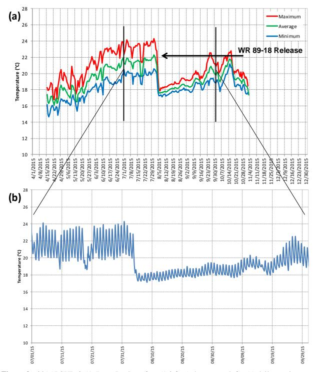
**Figure 9:** 2015 LSYR-0.51 (Long Pool) surface (1.0 foot) thermograph for (a) daily maximum, average, and minimum values and (b) hourly data for the period of 7/1/15 - 10/1/15.
