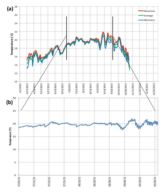
**Figure 35**: 2015 SC-3.0 (Highway 1 Bridge Pool Habitat) bottom (4.0 feet) water temperature for (a) maximum, average, and minimum for the entire period of deployment and (b) hourly measurements for the period from 7/1/15 - 10/1/15.
