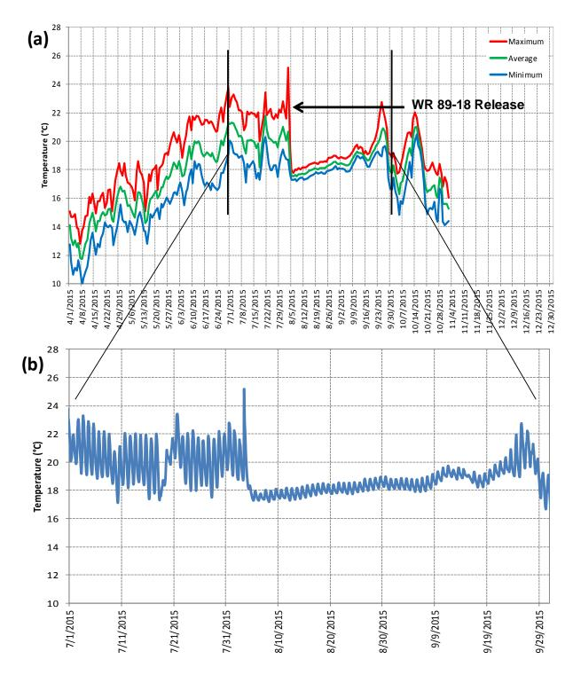
**Figure 8:** 2015 LSYR-0.25 (Downstream of the Stilling Basin) bottom (1.5 feet) water temperature for (a) daily maximum, average, and minimum for the entire period of deployment and (b) hourly measurements for the period 7/1/15 - 10/1/15.
