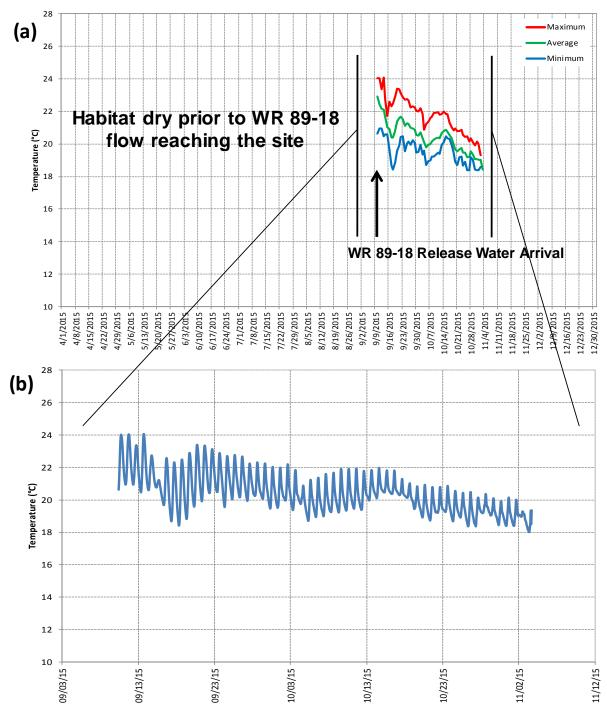
**Figure 20:** 2015 LSYR-8.7 (Head of Beaver Pool) middle (2.5 feet) thermograph for (a) daily maximum, average, and minimum daily values and (b) hourly data for the period 9/10/15 – 11/3/15; habitat unit was dry prior to WR89-18 releases.
