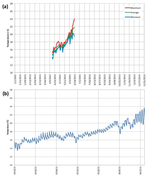
**Figure 39**: 2015 EJC-10.82 – water temperature at Rancho San Julian Fish Ladder bottom (2.5 feet) for (A) daily maximum, average, and minimum for the entire period of deployment and (b) hourly measurements for the period of deployment; the thermograph was removed from the habitat on 6/24/15 due to drying conditions.
