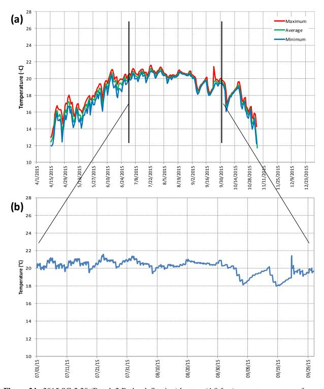
**Figure 34**: 2015 SC-2.20 (Reach 2 Bedrock Section) bottom (4.0 feet) water temperatures for (a) daily maximum, average, and minimum temperatures for the entire period of deployment and (b) hourly measurements for the period from 7/1/15 - 10/1/15.
