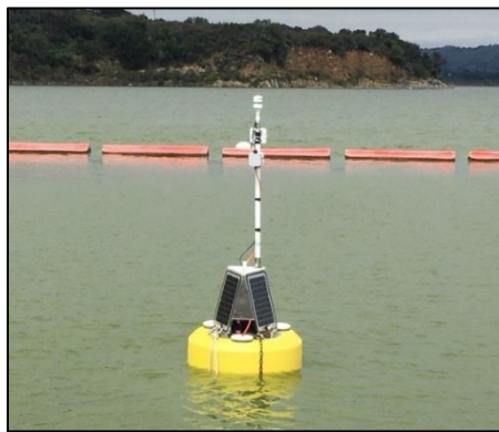
Lake Cachuma Water Quality Monitoring Buoy
