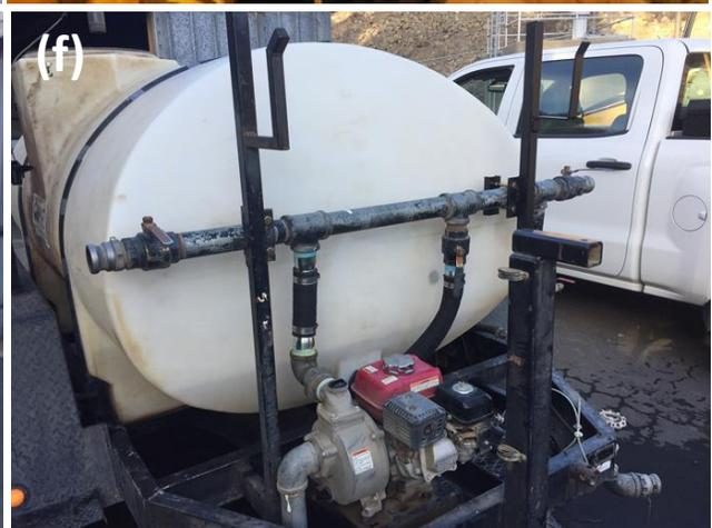
**Exhibit 1:** Water trailer maintenance showing (a) removal of tank, (b) new suspension welds, plastic welding (c) outside of the tank and (d) inside of the tank, (e) placing the tank on top of new trailer carpet, and (f) new hose and pipe connectors.
