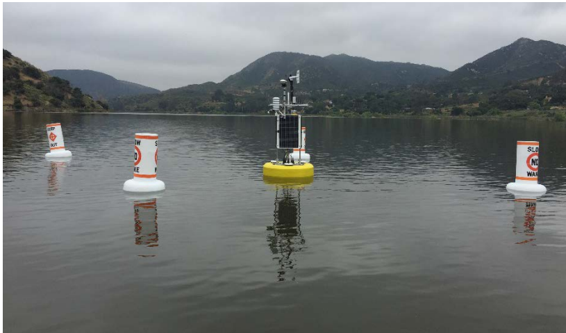
Figure 3: Picture of Lake Hodges, CA buoy-based weather station installed by DRI in 2017. Aerodynamic evaporation estimates are performed in-house at DRI and delivered via a web-portal in real-time.
