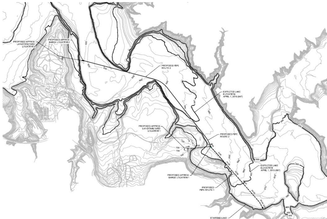
Figure 4. Drawing showing existing Pipeline, EPF Site 1 and PFSite 2. The final location of Site 2 is several hundred feet north of the location shown here, near the tip of the peninsula.
