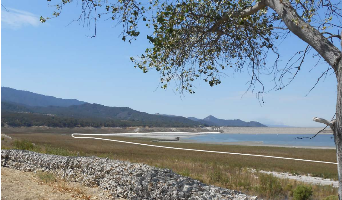
Figure 3. Portion of proposed alignment for Part 2 Pipeline. Much of this pipeline could be currently constructed on relatively dry lake bed.
