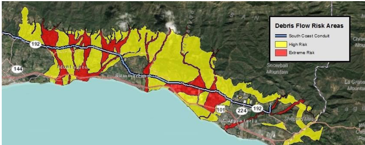
Figure 5-5. Debris Flow Risks for the South Coast Conduit
