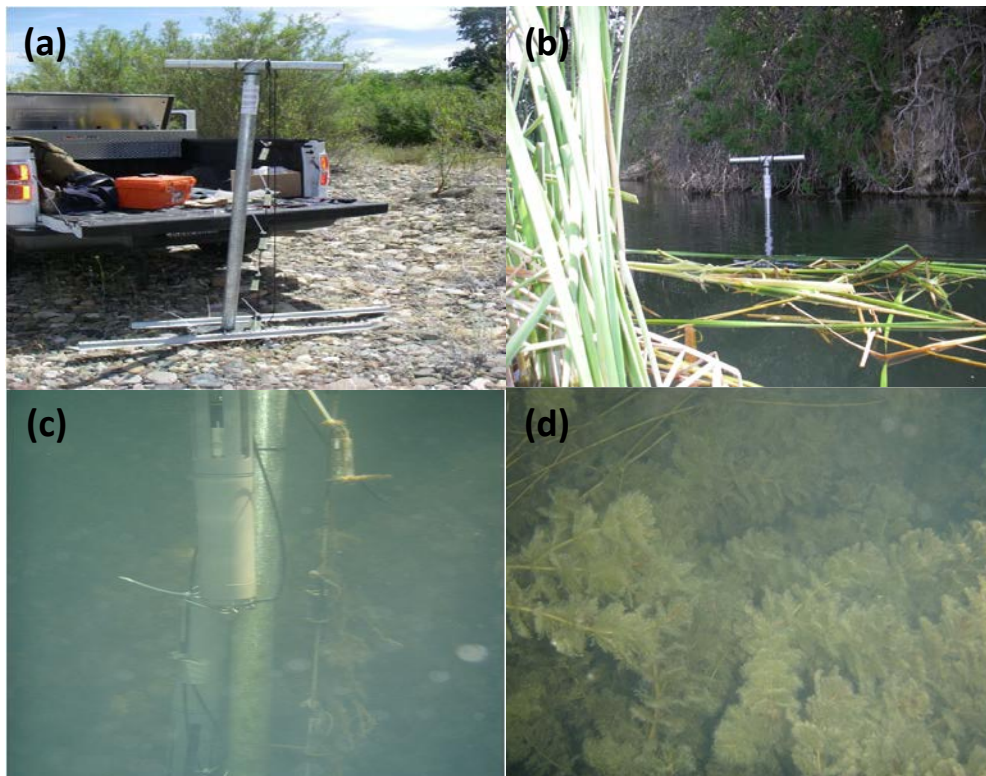
Figure 21: 2010 sonde vertical array at the Encantado Pool (LSYR-4.9) showing the (a) infrastructure prior to entering the water, (b) deployed infrastructure, (c) instruments underwater, and (d) aquatic vegetation on the bottom of the pool.
